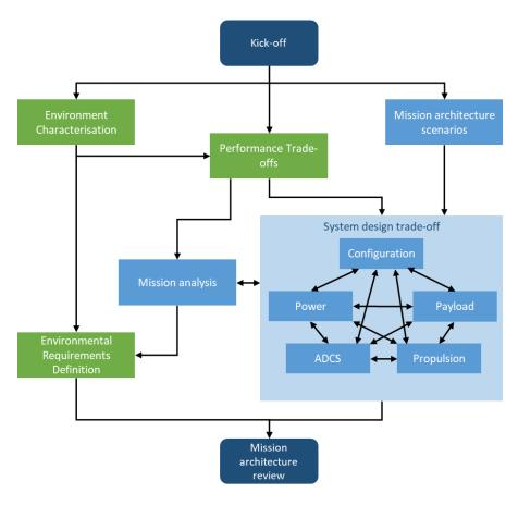
Figure 1: Systems Engineering process until mission architecture definition.
