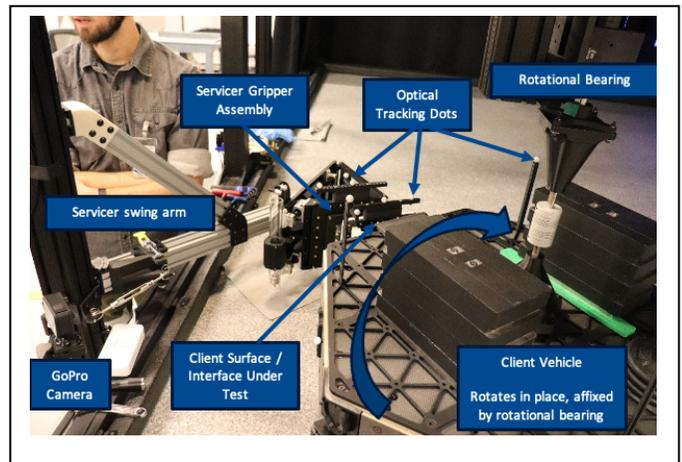
Fig. 7. Rotational air bearing test rig as assembled for testing
