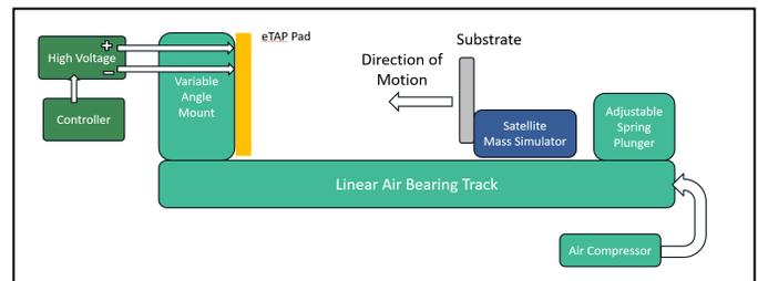
Fig. 4. eTAP™ 1D air track block diagram testing
