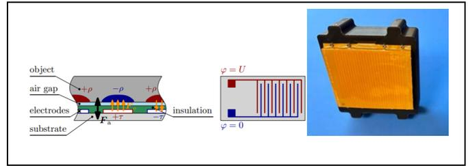
Fig. 1. Method of operation of eTAP™ gripper (left), and physical gripper (right)
