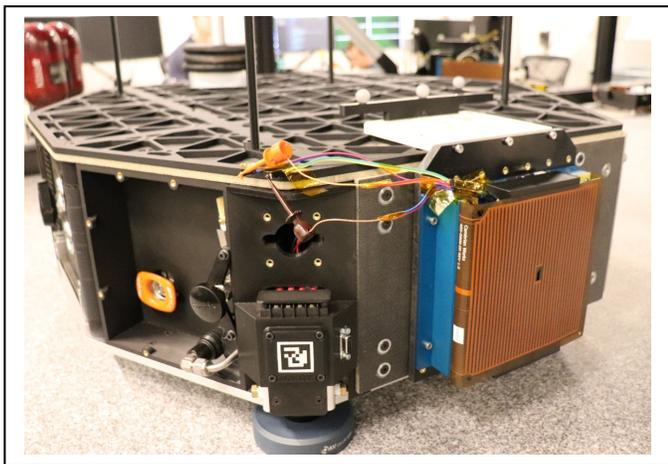
Fig. 6. eTAP™ Pad installed on air bearing craft
