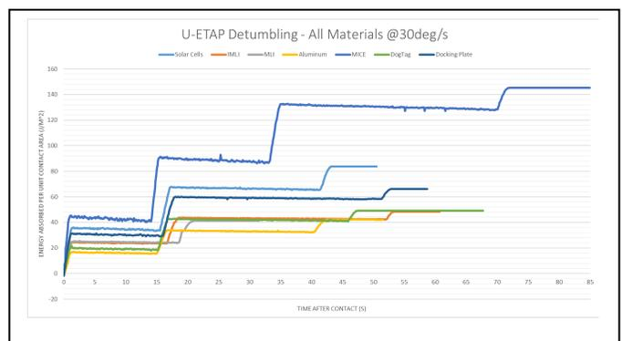
Fig. 8. Comparison of detumble performance across all materials, scaled for surface contact area
