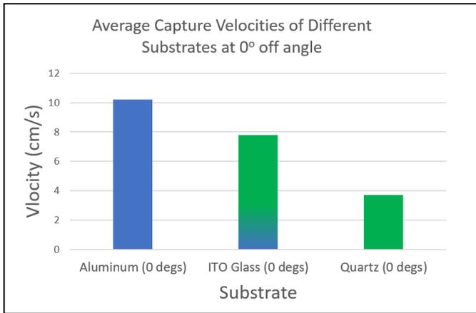
Fig. 5. eTAP™ 1D air track maximum capture velocities
