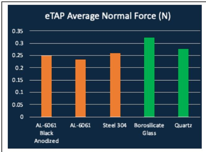
Fig. 3. eTAP™ Pad normal attachment force test results (ambient pressure)
