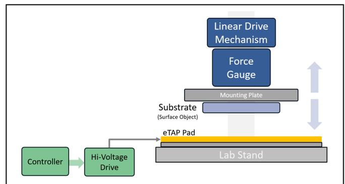
Fig. 2. eTAP™ Pad normal force test stand block diagram
