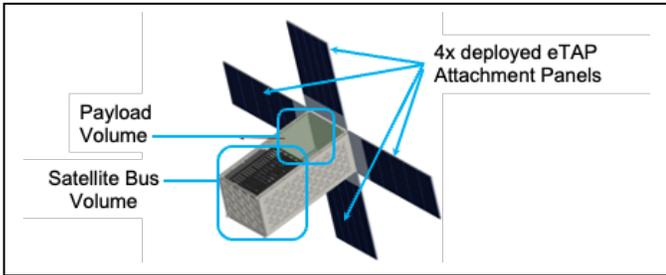
Fig. 9. SPIDEE-equipped 16U spacecraft with volume for additional payloads
