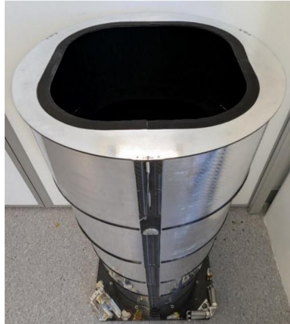
Figure 15 Deployed configuration of the baffle flight unit
