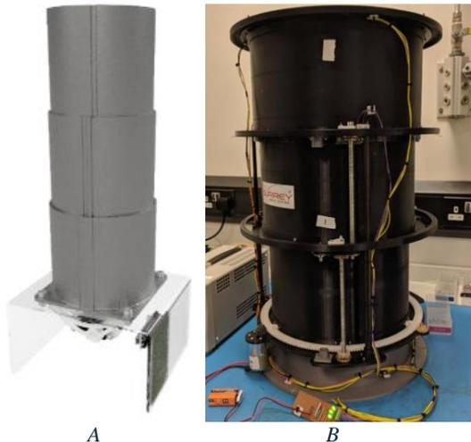
Figure 1 A) Deployable telescopic baffle demonstration model [4]. B) Breadboard model of a deployable barrel concept [12]
