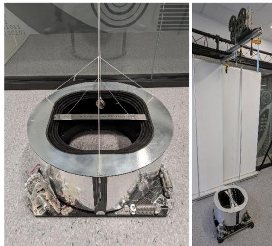
Figure 16 Functional deployment baffle test with off-loading passive mechanism
