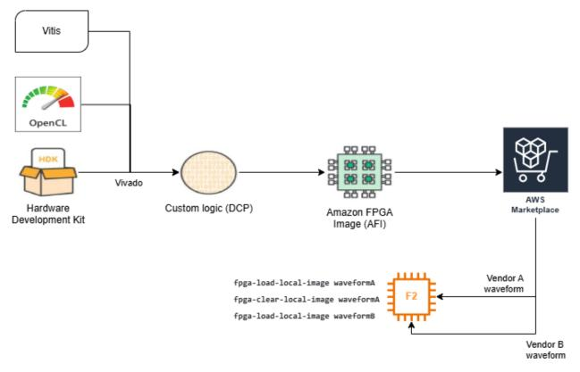
Fig. 3: Waveform orchestration with EC2 F2 FPGA
