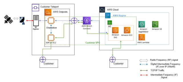
Fig. 2: Architectural diagram of a virtualized satcom system with SDR (de)modulation, (de)coding in AWS Cloud
