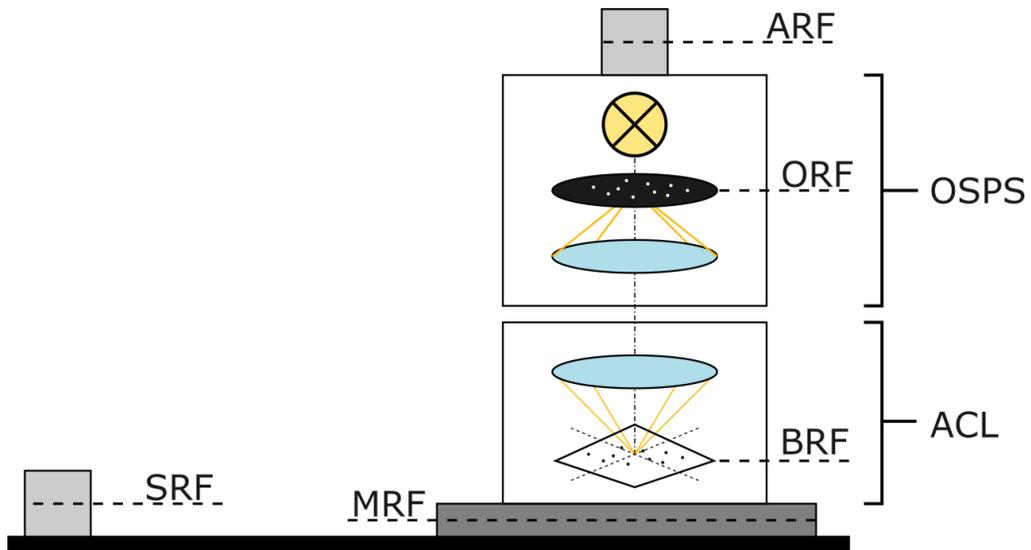
**Figure 4: Functional principle of the OSPS measurement, also showing the OSPS Reference Frame (ORF) and Alignment Reference Frame (ARF)**
