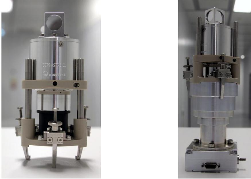
**Figure 3: OSPS - Alignment Tool (left), OSPS mounted on ASTRO© CL (right)**
