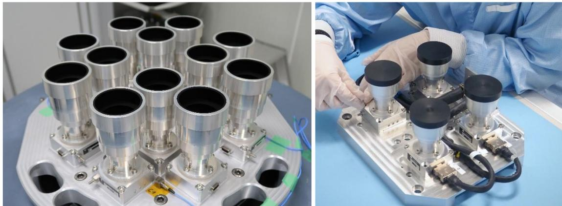
**Figure 2: Twelve ASTRO<sup>®</sup> CL on vibration test mount (left). Four ASTRO<sup>®</sup> CL in preparation for thermal testing (right).**
