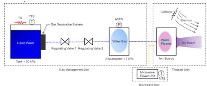
Figure 1 Schematic of PBI thruster
