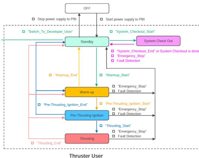
Figure 3 Mode transition diagram of PBI
