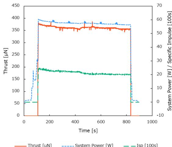
Figure 4 PBI operation test result on the ground. The temperature at the start point was 27 degrees of Celsius.
