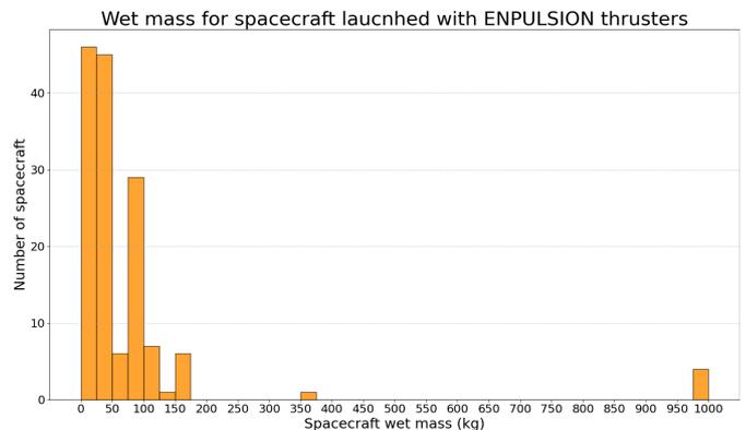
Fig. 4 Mass distribution of spacecraft using FEEP propulsion systems
