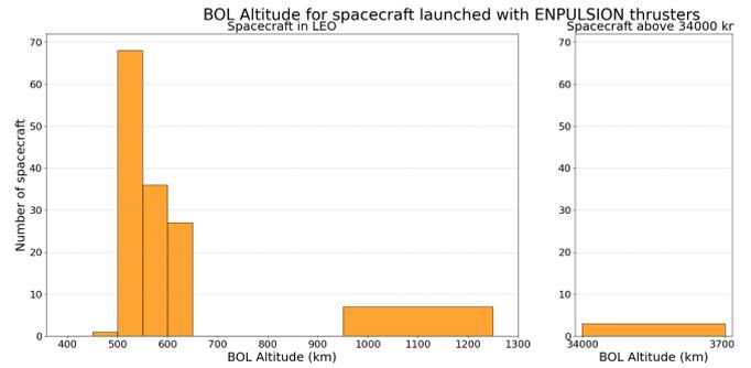
Fig. 3 BOL altitude distribution of spacecraft using FEEP propulsion systems
