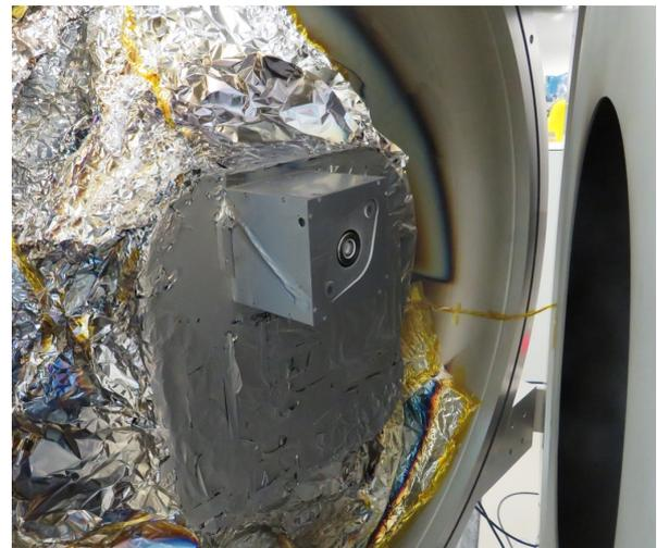
Fig. 7 NANO R<sup>3</sup> during thermal correlation testing housed within test enclosure which is mounted on the thermal interface system.
