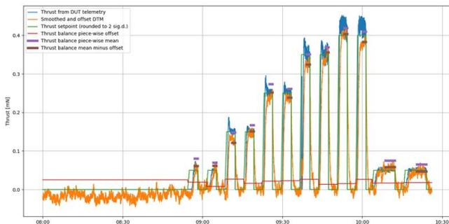
Fig. 6 Thrust measurements of the NANO R3 performed at FOTEC thrust balance comparing directly measured thrust to thrust calculated by the onboard electronics based on telemetry measurements [15].
