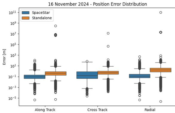
**Figure 17: Error distribution SpaceStar® and Standalone GNSS**
