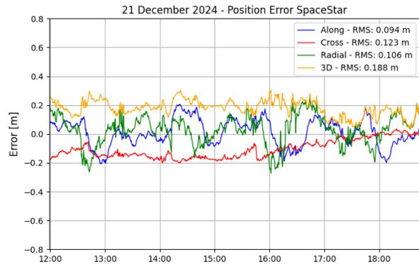
**Figure 11: Position error SpaceStar® using ESA reference orbits**
