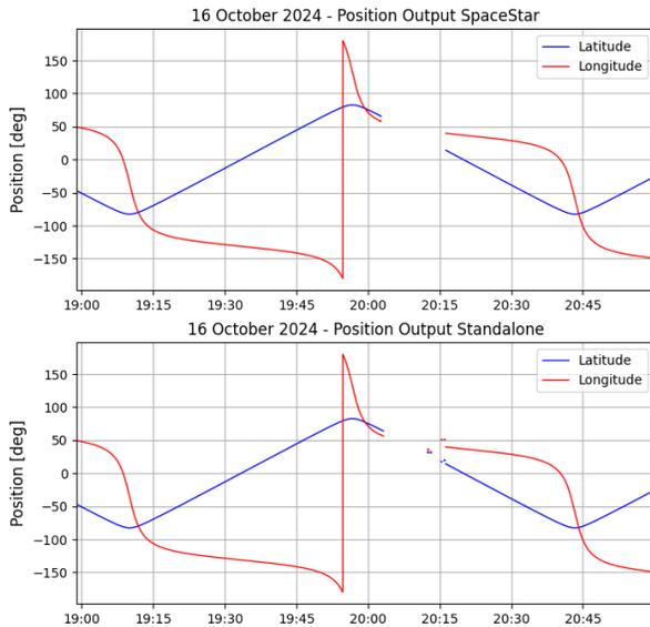
**Figure 18: Position output difference in presence of spoofing signals**
