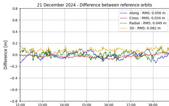
**Figure 13: Difference between ESA and Fugro reference orbits**
