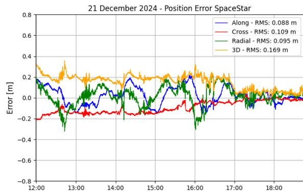
**Figure 12: Position error SpaceStar® using Fugro reference orbits**
