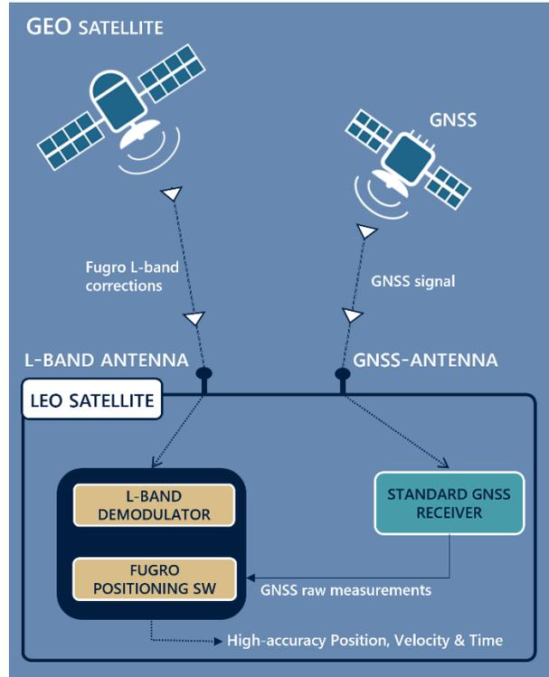
**Figure 4: SpaceStar® onboard architecture**
