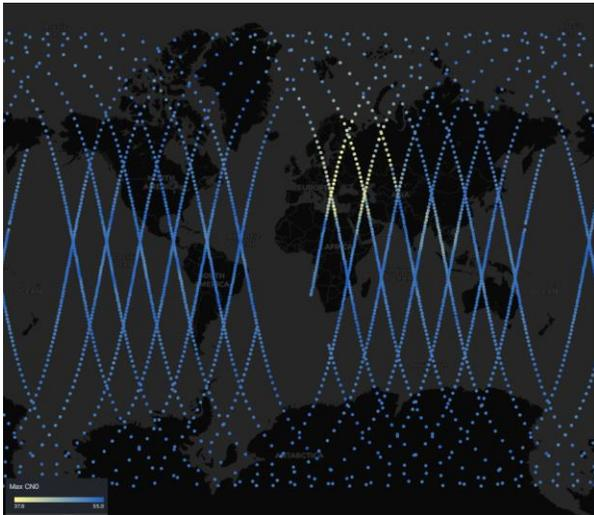
**Figure 15: Overlay of GNSS Max CN0**
