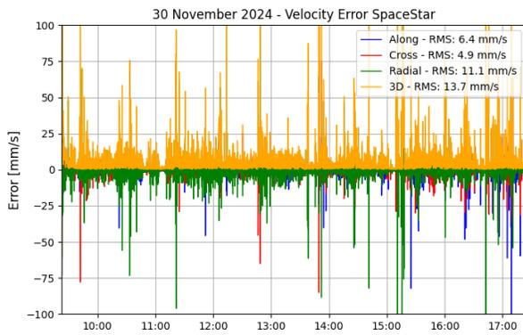
**Figure 6: In-orbit velocity results SpaceStar®**
