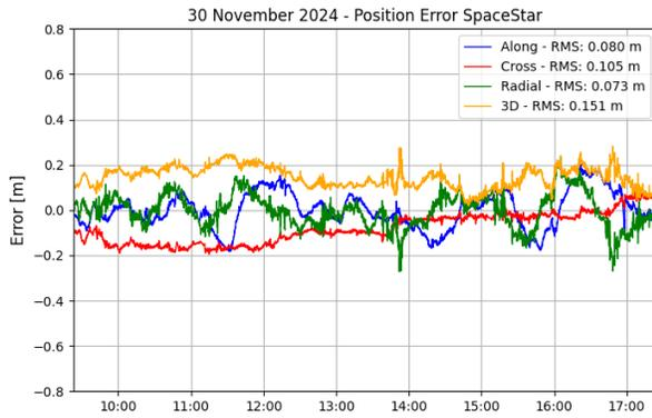
**Figure 5: In-orbit position results SpaceStar®**
