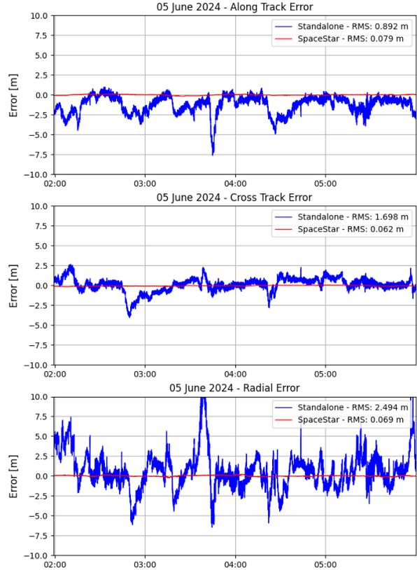
**Figure 8: Position comparison SpaceStar® and Standalone GNSS**
