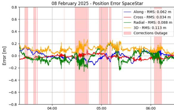
**Figure 14: SpaceStar® performance in presence of L-band outages**
