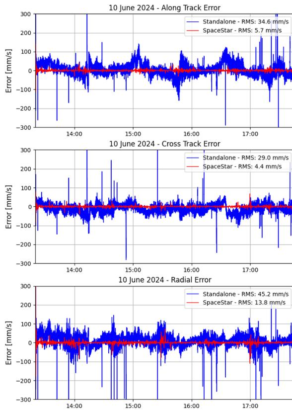
**Figure 9: Velocity comparison SpaceStar® and Standalone GNSS**
