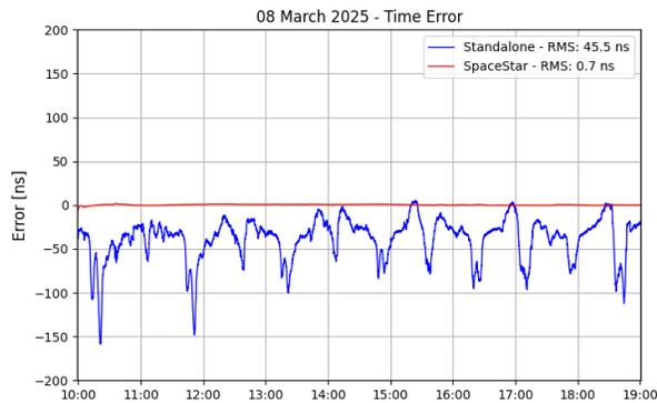
**Figure 10: Time comparison SpaceStar® and Standalone GNSS**
