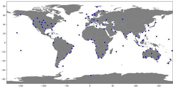
**Figure 1: Fugro reference receiver network used for GNSS multi constellation observations for generation of orbit/clock corrections**
