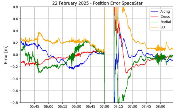
**Figure 16: SpaceStar® reconvergence after GNSS outage**
