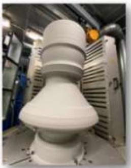
Figure 16: Cold sprayed In625 jacket on-top of Cu-alloy inner liner by ArianeGroup [9].
