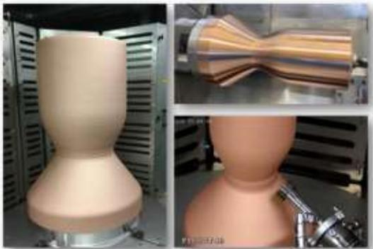
Figure 15: Cold spray of Cu-alloy – inner liner by ArianeGroup [9].
