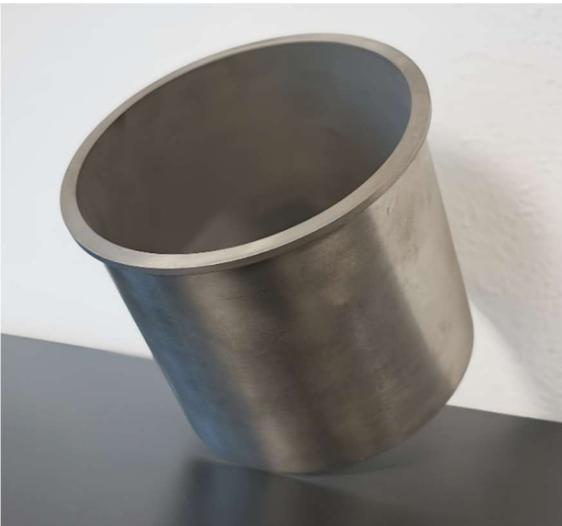
Figure 4: After mandrel removal and after post machining [13].
