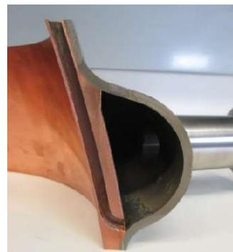
Figure 14: Inner structure of manifold [4].
