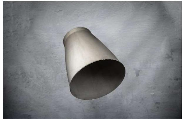
Figure 10: Final C-103 nozzle with Al mandrel removed, by chemical desolution [13].
