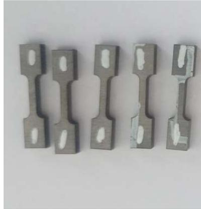
Figure 6: Five tensile specimens with heat treatment [13].
