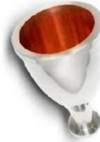
Figure 12: Rocket nozzle after machining – manufactured by Impact Innovations [4].
