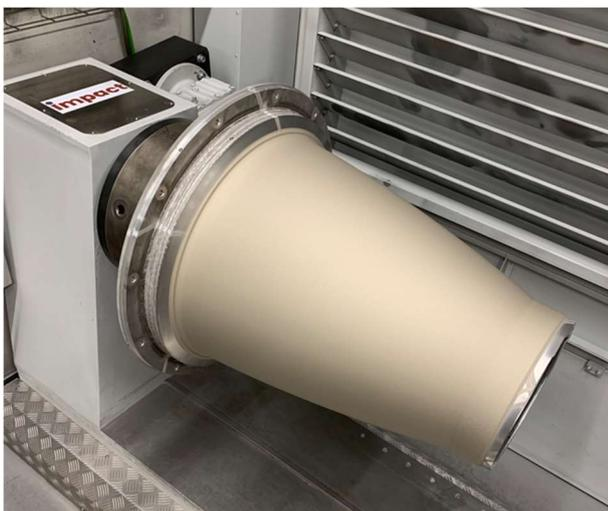
Figure 9: Finished cold sprayed C-103 nozzle on Al mandrel [13].
