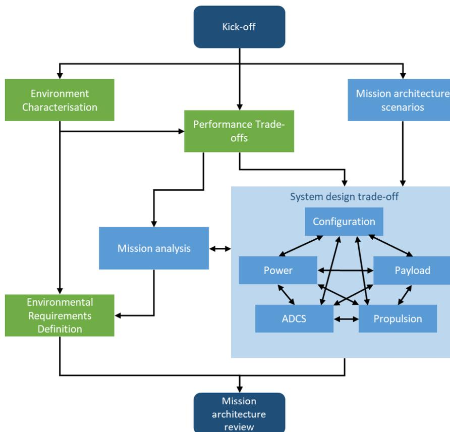
Figure 1: Systems Engineering process until mission architecture definition.
