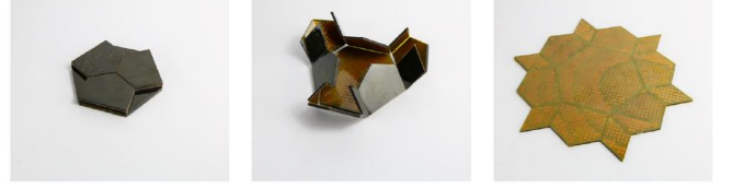
Figure 2: Hexagonal twist RA prototype using panels and flexible hinge mechanism. The deployment sequence presented from left to right.
