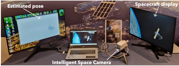
Fig. 1. Spacecraft pose estimation executing directly on the Intelligent Space Camera. Camera captures frames of scene on right-hand monitor, and streams position and pose estimates directly to the laptop for display on the left-hand monitor.
