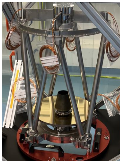
Fig. 14. Metering Structure, Optical Tube Assembly
