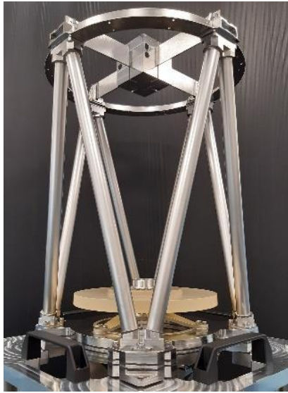
Fig. 6. Primary Truss Structure
