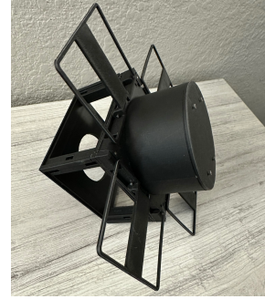
Fig. 6. A photograph showing the first implementation of Chickadee mechanical housing with four deployable wings that can carry solar cells to support its necessary functions.
