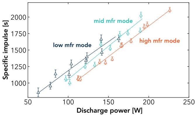
Fig. 4. Specific impulse versus discharge power.
