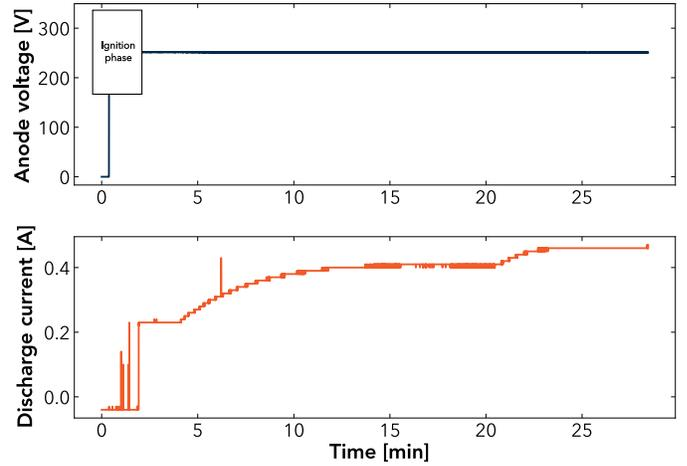
Fig. 2. Instance of discharge telemetry profile. (top) Anode voltage, (bottom) anode current.
