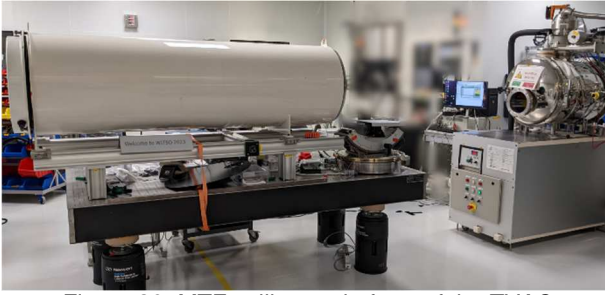
Figure 20. MTF collimator in front of the TVAC
