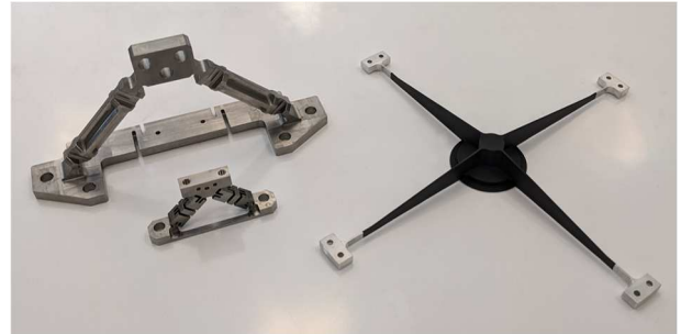
Figure 9. Bipods flexures and external baffle extra obscuration
