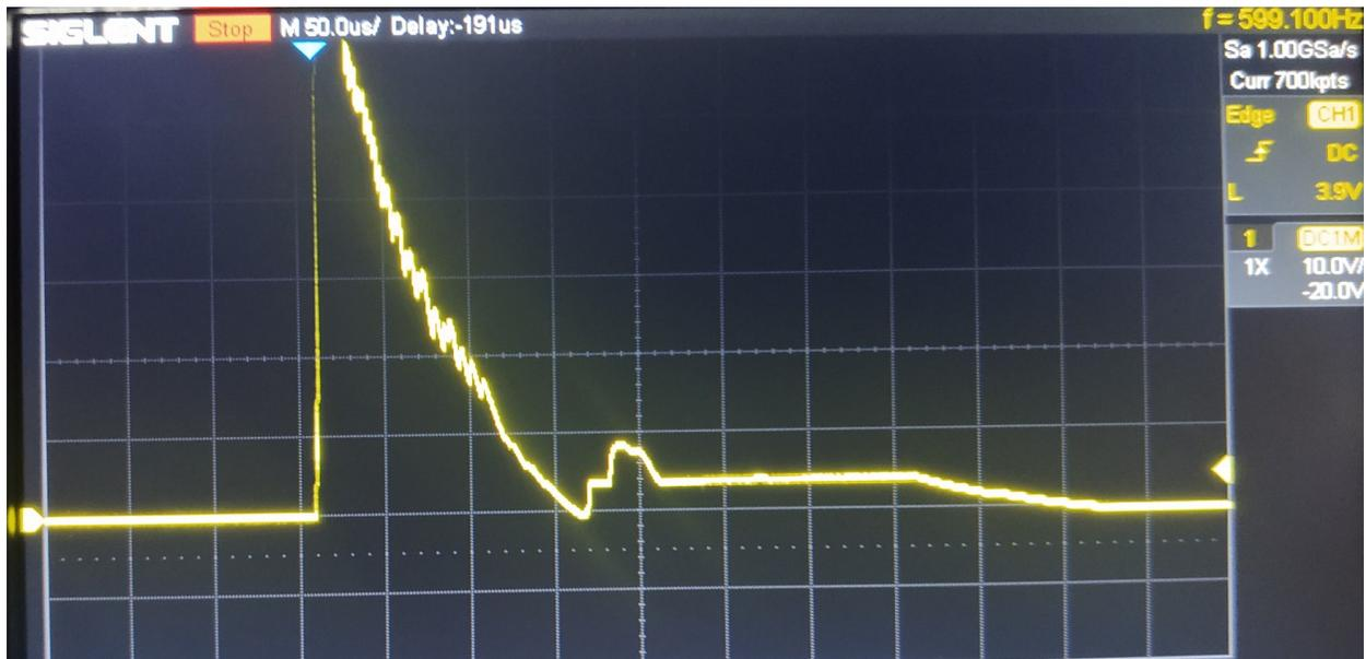
Figure 22 Single gamma pulse using boronated water. Note secondary pulses during the decay period.
