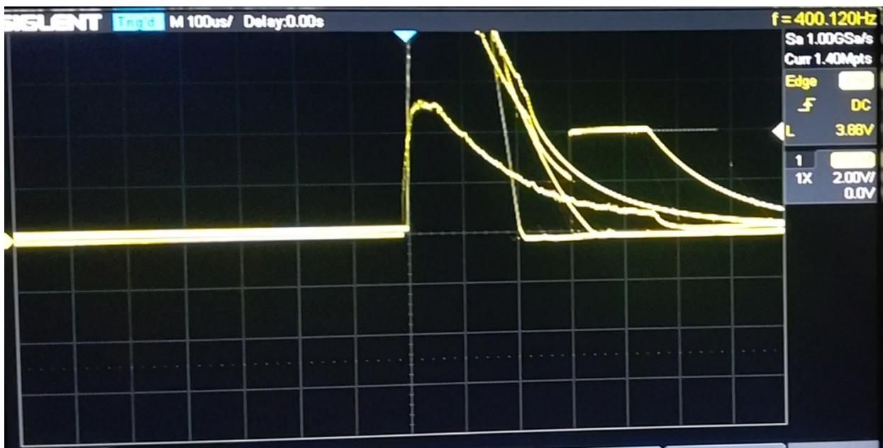
Figure 21 Multiple gamma pulses using boronated water
