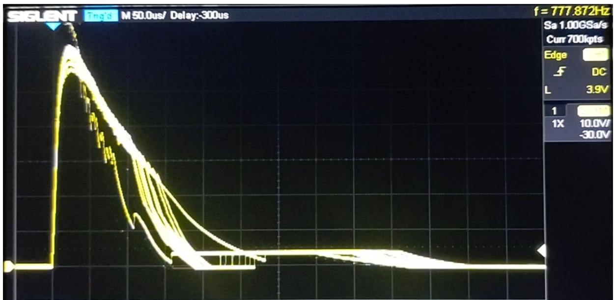
Figure 23 Multiple pulses using boronated water and higher acceleration voltage. Note increased frequency and strong secondary pulses.
