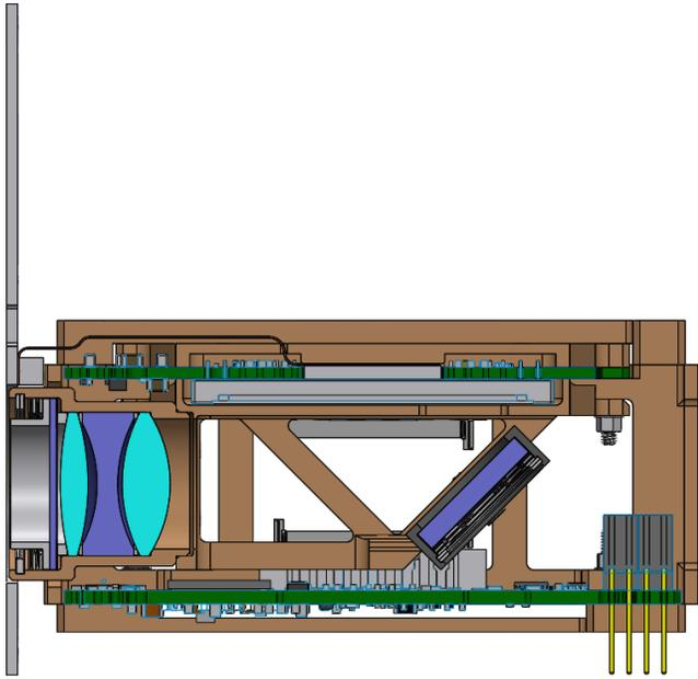
Fig. 4. LUVCam payload cut view
