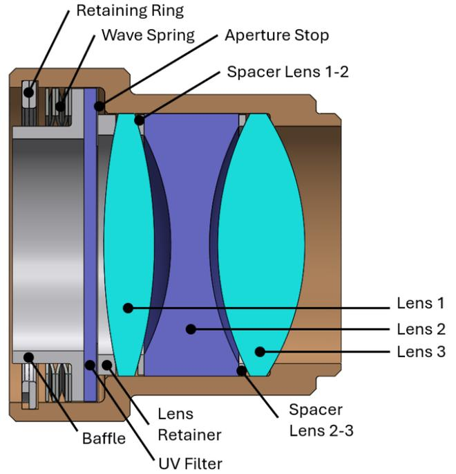
Fig. 5. LUVCam,s telescope cut view
