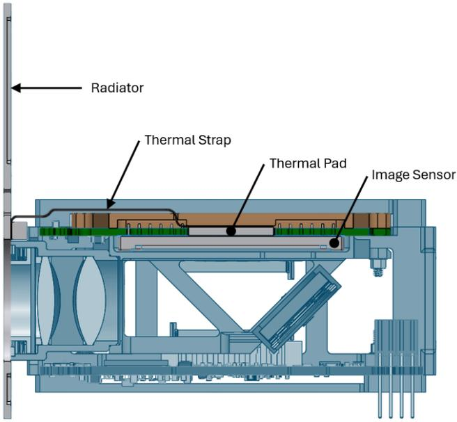
Fig. 6. Thermal path from the image sensor to the radiator
