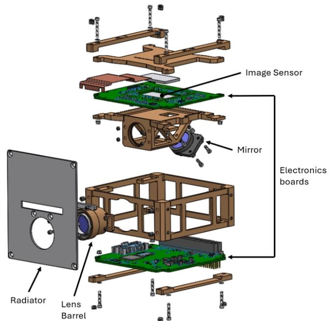
Fig. 3. LUVCam payload exploded view
