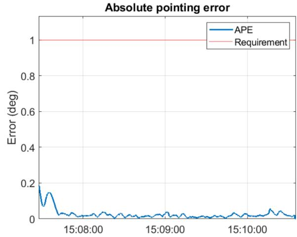
Fig. 6. Absolute pointing error achieved with orbital mode.
