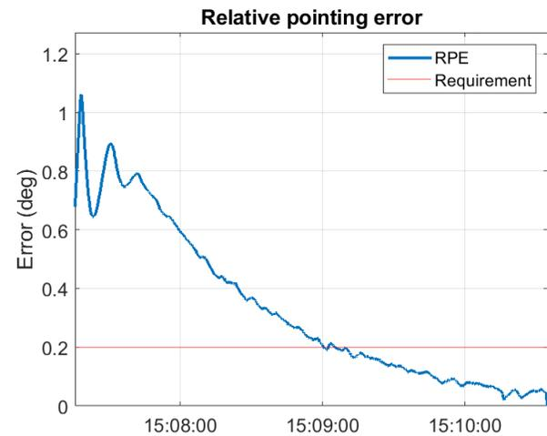
Fig. 7. Relative pointing error achieved with orbital mode.
