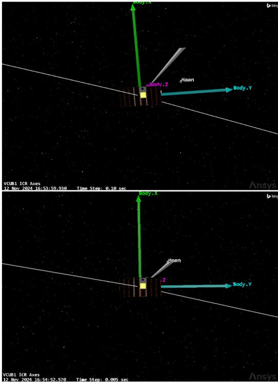
Fig. 12. Pointing profile for moon imaging, first commanded offset (above) and the pushbroom (below).
