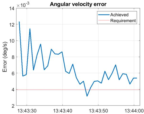
Fig. 9. Angular velocity error achieved during imaging.
