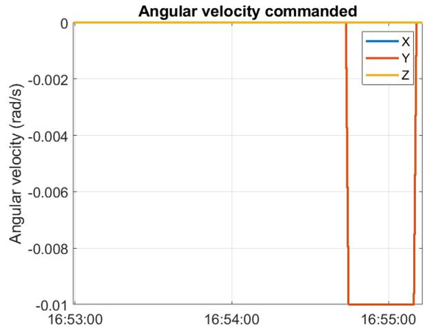
Fig. 15. Angular velocity commanded during Moon imaging.
